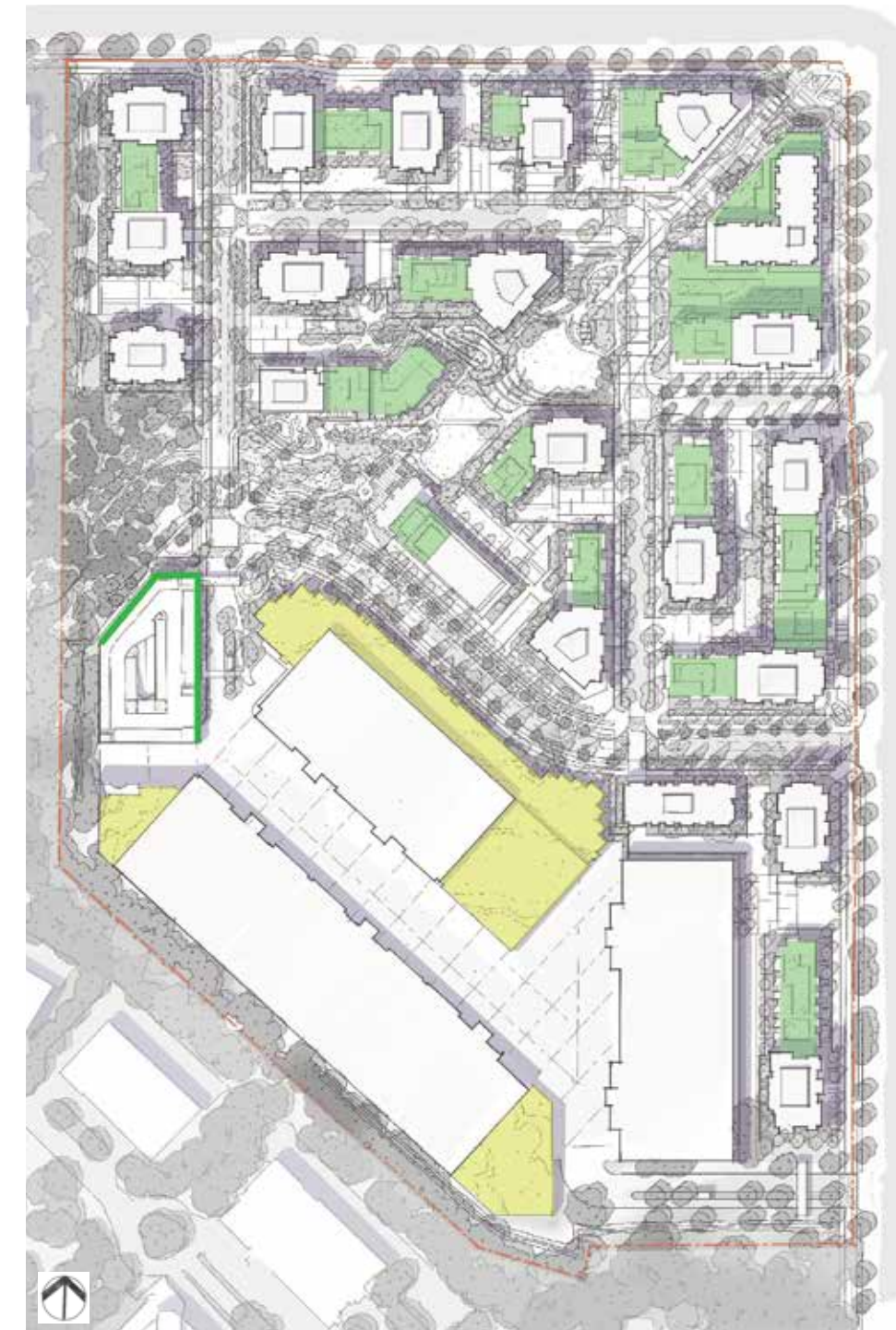
FIGURE 6-72: GREEN ROOFS DIAGRAM
